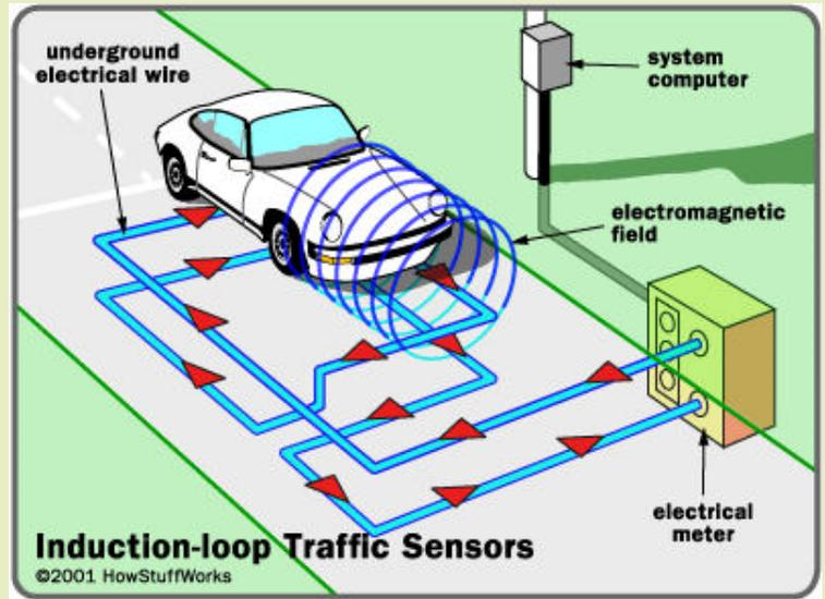
This graphic by [www.HowStuffWorks.com](http://www.HowStuffWorks.com) shows the mechanics of an induction-loop traffic sensor.
