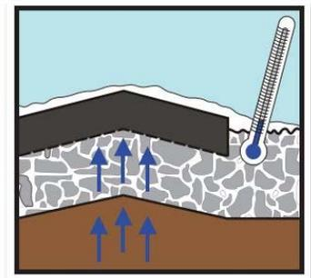
The moisture freezes when temperatures drop, causing the ground to expand and push the pavement up.
