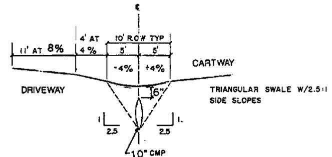
DEEPEN SWALE IN LOWER REACHES OF WATERSHED TO ACCOMMODATE 12" DRAIN PIPE UNDER DRIVEWAY.
