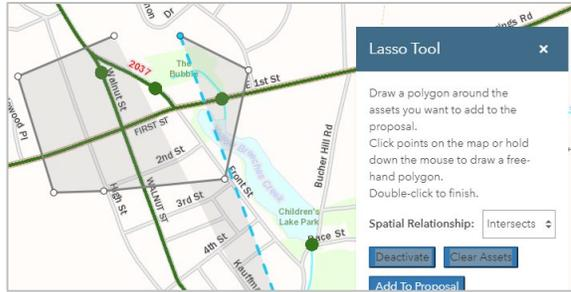
When the polygon is completed the selected roads/bridges will be highlighted.
