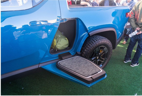
FIGURE 1.3 The Rivian R1T gear tunnel offers a slide-out platform for easy access storage and to increase usable space.
