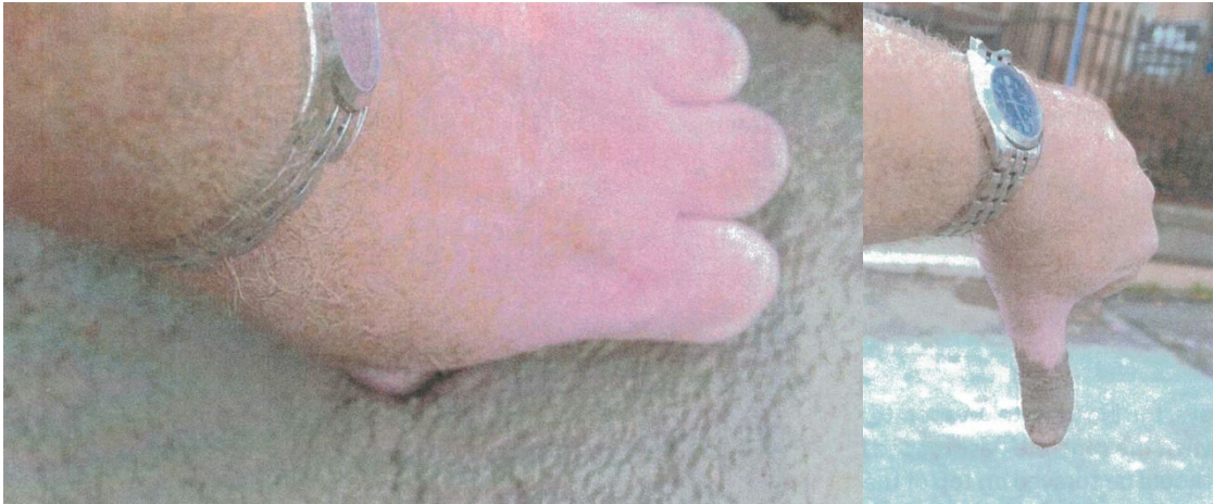
Figure 11. The “thumb test” to check whether concrete has sufficiently set to begin finishing (from: [8])
