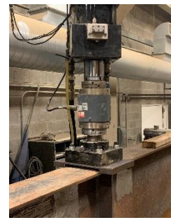
b) Fatigue conditioning of girder Ends B using 50 kip capacity servo-hydraulic actuator
