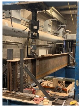
b) Fatigue conditioning of girder Ends B using 50 kip capacity servo-hydraulic actuator
