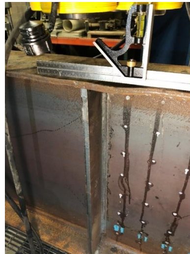
b) distortion of top flange associated with web yield under point of application of load
