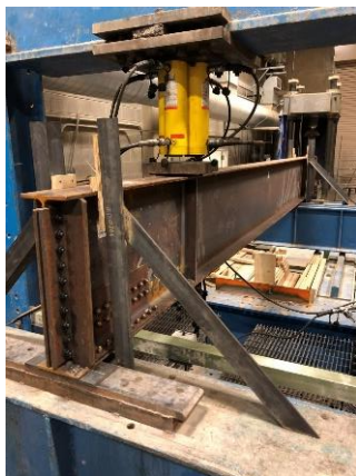
a) Monotonic tests of girder Ends A and B using four 70 kip capacity hydraulic cylinders
