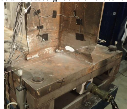
c) end region of damaged specimen following testing showing crippling of web and stiffeners
