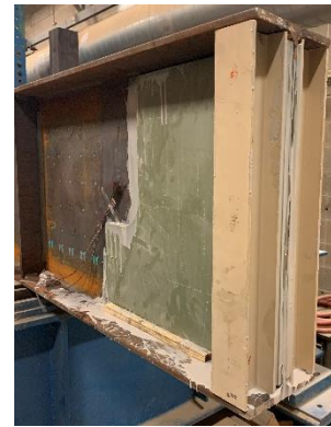
completed FRP repair
