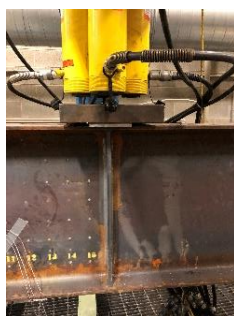
a) Monotonic tests of girder Ends A and B using four 70 kip capacity hydraulic cylinders
