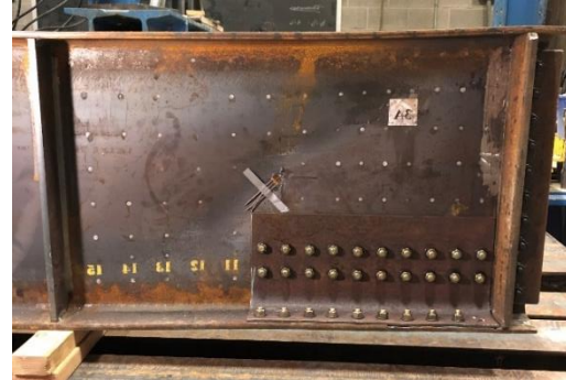
b) observed behavior following testing (image mirrored)
