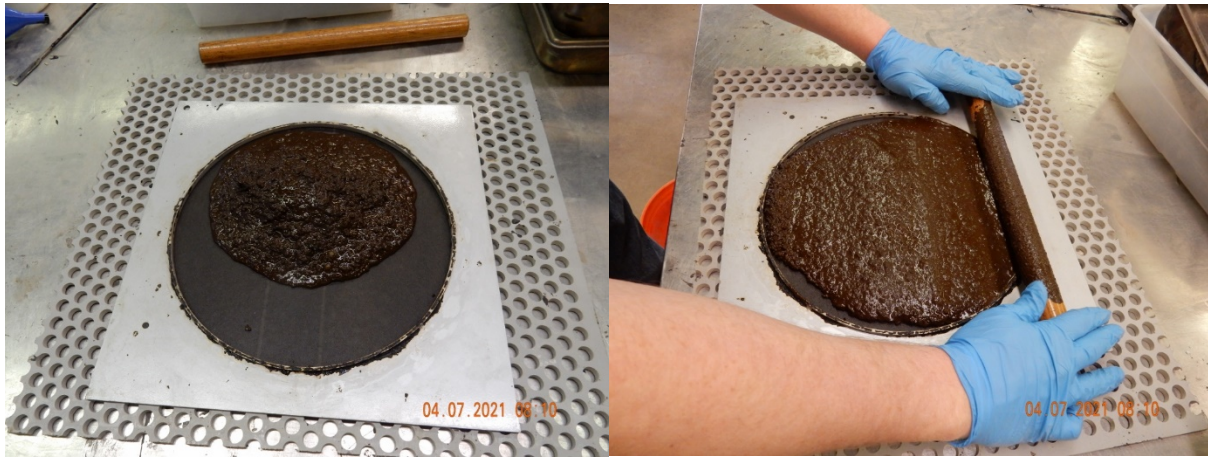
Figure 27. (a) The micro surfacing material poured into the mold, (b) spreading the micro surfacing material using the wooden dowel rod to evenly spread across the mold to uniform thickness.
