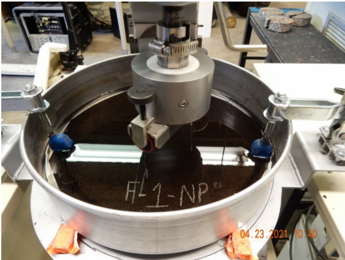
Figure 28. Micro surface specimen clamped in the abrasion pan with the pan filled with water before testing.
