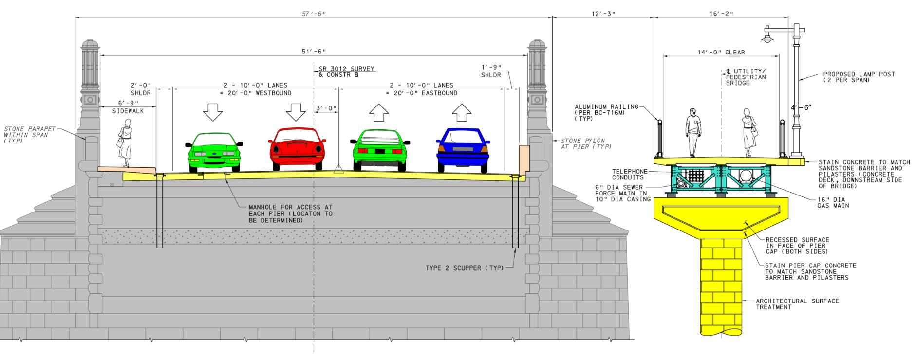
PROPOSED TYPICAL SECTION AND PIER ELEVATION
